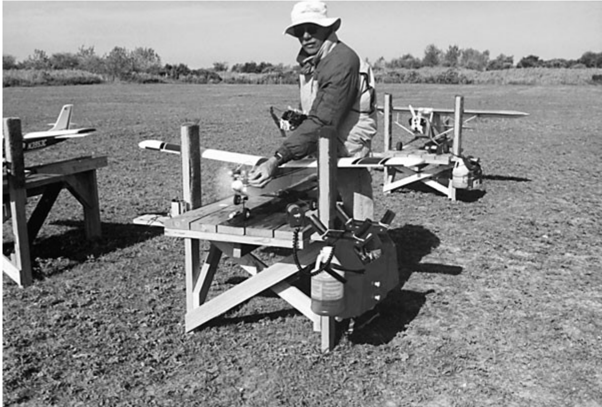
Charlie Meyer demonstrates the use of the bench while adjusting the needle valve from behind the propeller. There's no need to lean over to pick up the model!
